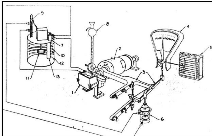
**Figure 1. Diagram of the basic parts of the farinograph**
